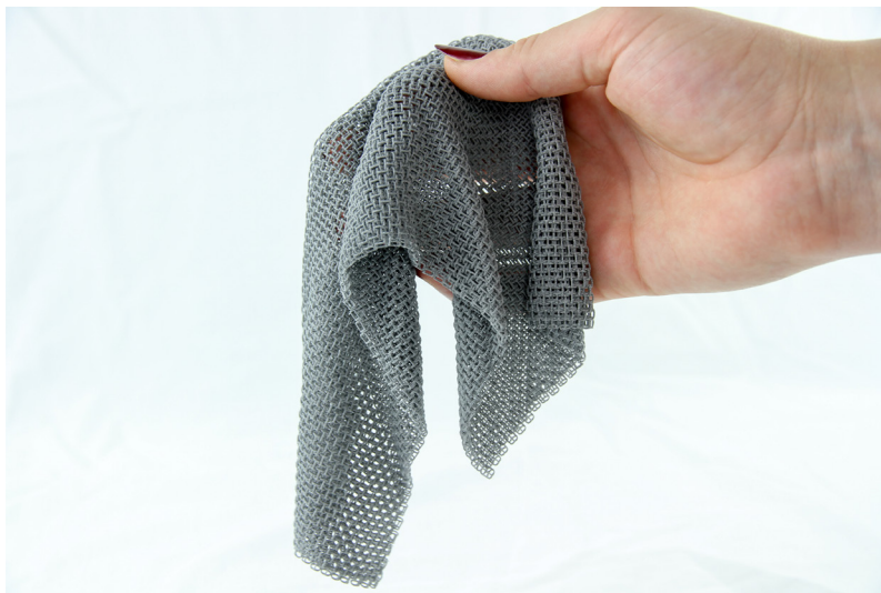
Image 1 - Multiple small intersecting joints that are printed together to form a fabric like texture.
