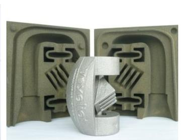
12. Casting with sand mold
